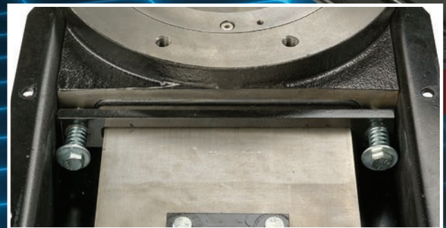
Spring-loaded packing option
