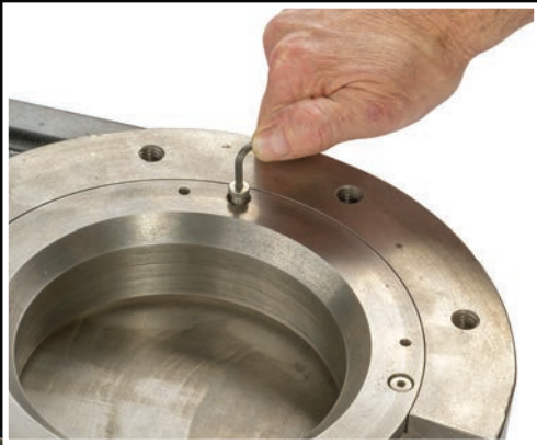
Easy replacement seal bolts
